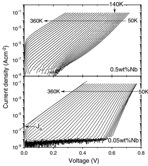
**Figure 3.** Semi-log plot of the characteristics of LCMO/STON (0.5 wt%Nb) (top panel) and LCMO/STON (0.05 wt%Nb) (bottom panel) measured under different temperatures below 360 K.
