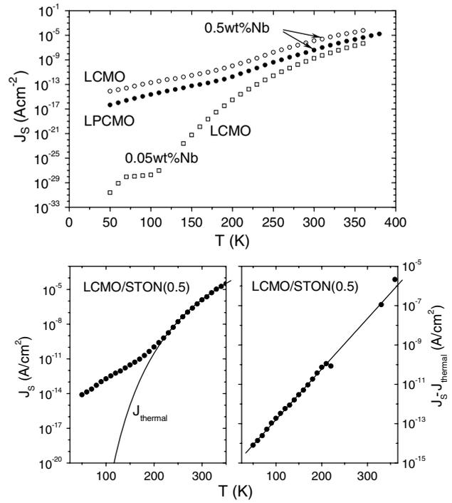
**Figure 4.** Top panel: temperature dependence of saturation current  $J_s$  derived from the current–voltage characteristics of the junctions. Bottom panel: thermal current ( $J_{\text{thermal}}$ ) and tunnelling current as functions of temperature. The former is described by the equation  $J_s \propto T^{3.5} \exp(-qV_D/k_B T)$  with  $V_D = 0.48$  eV, and the latter by  $J_s - J_{\text{thermal}} \propto \exp(T/T_0)$  with  $T_0 \approx 17.24$ .
