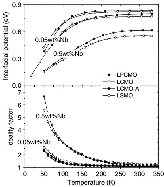
**Figure 5.** Top panel: built-in voltage as a function of temperature for the manganite junctions with different tolerance factors. Bottom panel: ideality factor of the manganite junctions. LCMO-A denotes the LCMO/STON (0.05 wt%Nb) junction annealed at 600 °C in air for 1 h.
