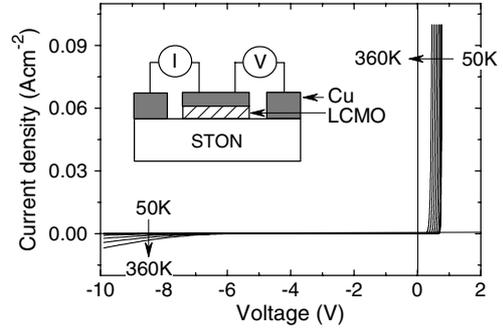
**Figure 2.** Current–voltage characteristics of the manganite junction LCMO/STON (0.05 wt%Nb) measured under different temperatures below 360 K. Inset plot is a schematic diagram showing the electrode setting.
