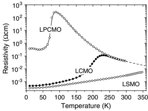
**Figure 1.** Temperature dependence of the resistivity of the manganite films with different tolerance factors. The dashed line is a guide for the eye.
